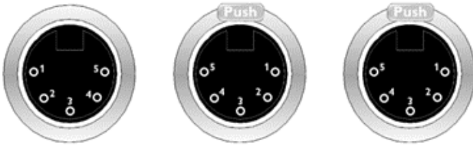
DMX in (male) DMX thru (female) DMX out (female)
